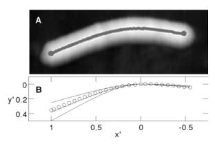
Figure B shows where the mechanical equations for beam bending for a beam under uniformly distributed force are fit to the shape of the TMV found with the medial-axis software. This fit yields the ratio of distributed frictional force to the bending rigidity of the TMV.
