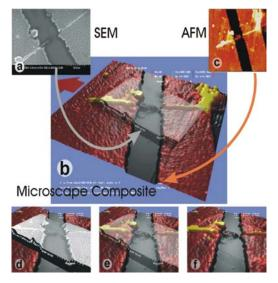
The image to the right shows the overview of AFM and SEM scans of the same area, a carbon nanotube that was draped between two raised electrodes and then broken. The simplest combination of the two data sets is shown here: the data sets were aligned by hand and the SEM laid over the underlying AFM topography using projective texture mapping. The user can adjust the relative mixture of the two data sets.
