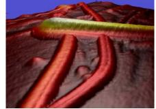
where one tube was pushed end-on to slide over another pair of tubes; the AFM probe was then carefully inserted by feel between the first two tubes to peel them apart – leaving the third tube suspended between them.
